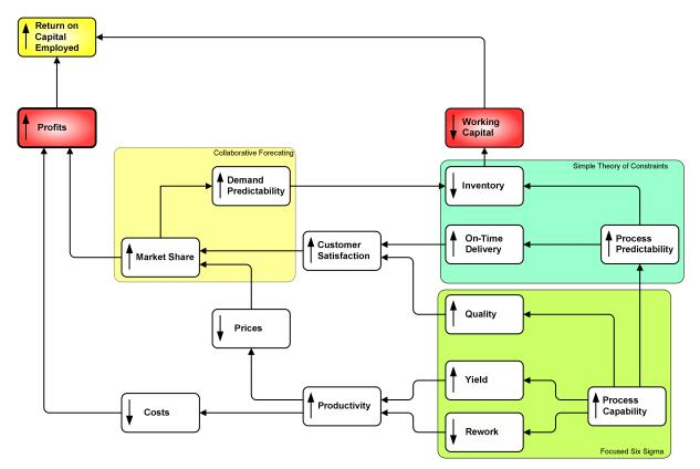
**Figure Two:** Manufacturing Cause and Effect: How Six Sigma and Theory of Constraint Applies. (Shannon 2003).
